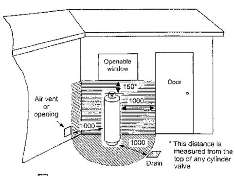
Shading indicates prohibited area for a drain or opening
